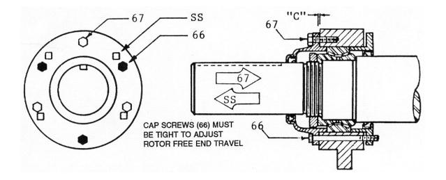
Loosen the cap screws and move the rotor toward the idle end by using the four set screws (SS) in the bearing cap. When the rotor touches the idle end cone measure the gap "C" again between the bearing cap and bearing housing. Rotor free end travel is equivalent to the difference between the two measurements.
