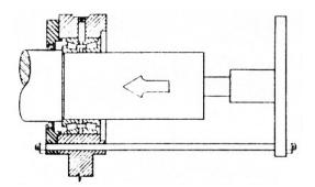
Using two slings and a pipe extension, work the shaft and rotor assembly out of the body through the idle end of the pump.
