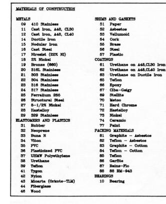
THIS PARTS LIST REFERS TO DRAWING NO. SV-686PL-1 AND PERTAINS TO PUMP MODELS SV-808, 1211, 1414, 1818, and 2023. COMPLETE PUMP MODEL DESIGNATION FOR A SPECIFIC
