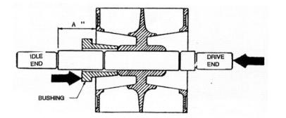
Make up a bushing, with a groove so as to miss the shaft key, for pressing against the rotor hub. Do not apply force other than at rotor hub. Do not attempt to remove the key from the shaft. Check dimension "A" before removing shaft:
