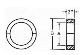
Remove the six cap screws holding the idle end bearing cap (19). Remove cap and adjusting shims (57) and alternating gaskets (55). Remove shaft nut and lock ring (45, 46). The steel inner bearing cap (17) will serve as a bearing pusher when set up with the split ring as show below.
