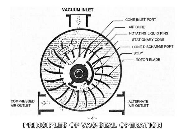
The patented Somarakis Vac-Seal is used with both liquid ring vacuum pumps and compressors. The pump or compressor will operate drop-tight around the shaft with no external leakage of sealant.
