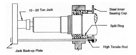
It is not necessary to remove the steel bearing housing (16) unless it has been damaged and requires weld repair and machining; leave it fastened to the head. The bearing housing requires no shims if removed and reinstalled.
